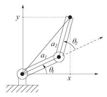
b. When solving the inverse Kinematics for the planar 2 link arm in the above image, explain under which conditions you can find: one solution, two solutions, no solutions, or infinite solutions.
