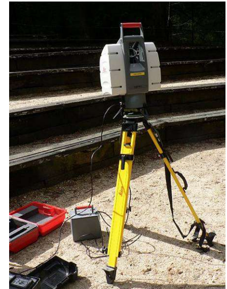
Leica terrestrial lidar (light detection and ranging) scanner
