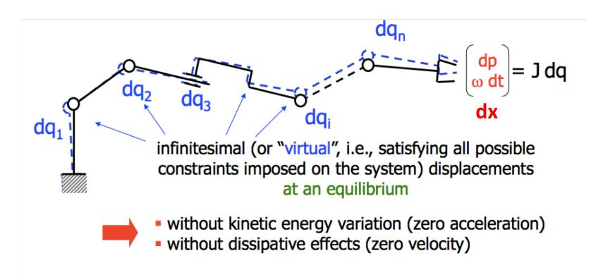
the "virtual work" is the work done by all forces/torques acting on the system for a given virtual displacement
