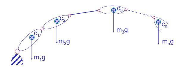
$$G = -(J_{v_1}^T(m_1g) + J_{v_2}^T(m_2g) + \dots + J_{v_n}^T(m_ng))$$
