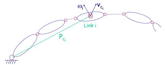
$$\frac{1}{2}\dot{q}^{T}M\dot{q} = \frac{1}{2}\dot{q}^{T}\left[\sum_{i=1}^{n}\left(m_{i}J_{v_{i}}^{T}J_{v_{i}} + J_{\omega_{i}}^{T}I_{Ci}J_{\omega_{i}}\right)\right]\dot{q}$$
