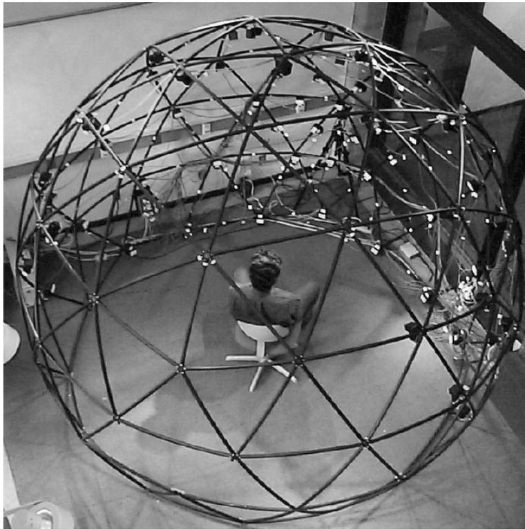
Figure 10: A geodesic dome with 64 strobes used to gather images under variable illumination and pose.
