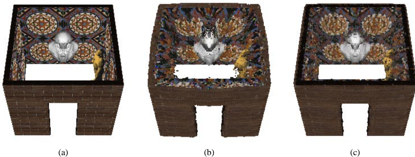
Fig. 13: Views of the reconstruction from far away camera viewpoints. (a) shows a rendered top view of the building, (b) the same view of the reconstruction, and (c) a new reconstruction resulting from adding image (a) to the set of input views. Note that adding a single top view drastically improves the visual quality of the reconstruction.
