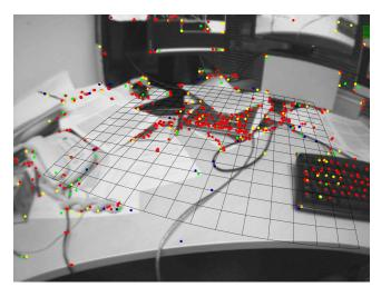
Figure 1: Typical operation of the system: Here, a desktop is tracked. The on-line generated map contains close to 3000 point features, of which the system attempted to find 1000 in the current frame. The 660 successful observations are shown as dots. Also shown is the map's dominant plane, drawn as a grid, on which virtual characters can interact. This frame was tracked in 18ms.
