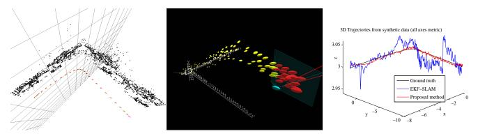
Figure 5: Comparison with EKF-SLAM on a synthetic sequence. The left image shows the map produced by the system described here, the centre image shows the map produced by an up-to-date implementation of EKF-SLAM [30]. Trajectories compared to ground truth are shown on the right. NB. the different scale of the z-axis, as ground truth lies on z=3.
