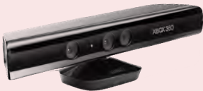
Kinect camera: Real-time depth measurement
