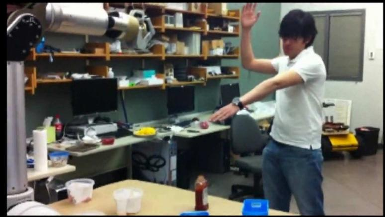
The human by pointing instructs the robot which ingredients are to be placed on the pizza
