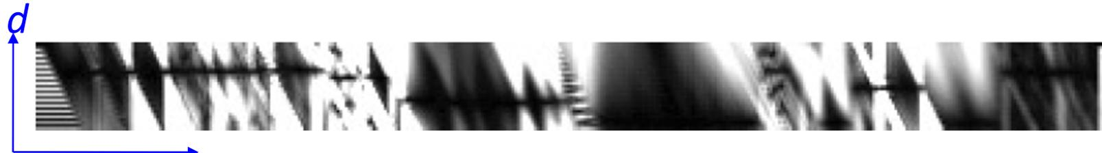
Simple pixel  $\neq$  window matching: choose the minimum of each column in the DSI independently:
