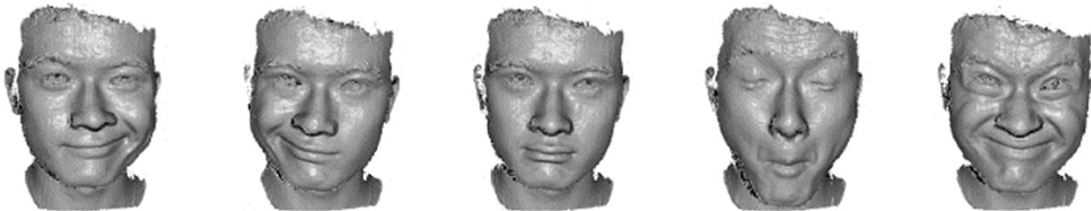
Spacetime stereo reconstruction with  $9 \times 5 \times 5$  window
